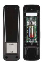
The B-PUPILLA XP20D adjustable photocell has a 12/24V receiver power supply and traditional or battery operated transmitter power supply. It avoids having to lay a cable to the transmitter (battery) and features selectable channels which allows the installation of up to 4 pairs of photocells and protection from interference produced by external light sources (such as vehicle LED headlights).
